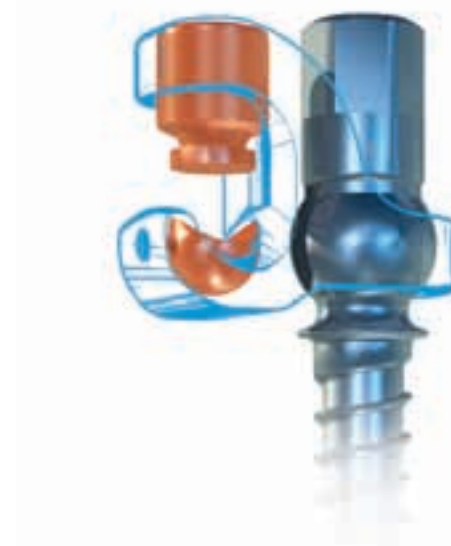
2. Independent locking of the rod in the screw head using the set screw.
